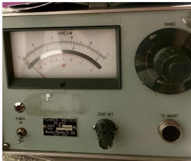
Anritsu ML81A power meter for mm-wave sensors. Makes a strange noise.
